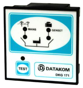
The DKG-171 provides a TEST mode pushbutton allowing the genset to be tested without a mains failure. The Test mode is also called Emergency Backup mode which keeps the genset running and makes a quick transfer in the event of a mains failure.
