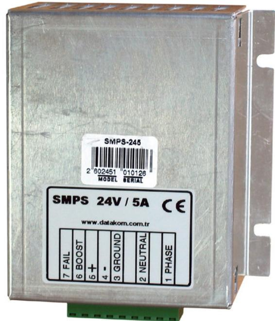
The units provide a "boost charge" input as a standard feature. When this input is pulled to battery negative, the output voltage of the charger will be set to the boost charge voltage. This feature may be used temporarily to improve battery life.
